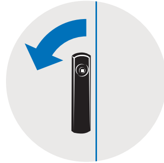
LH Door with escutcheon Opening direction is counter-clockwise
